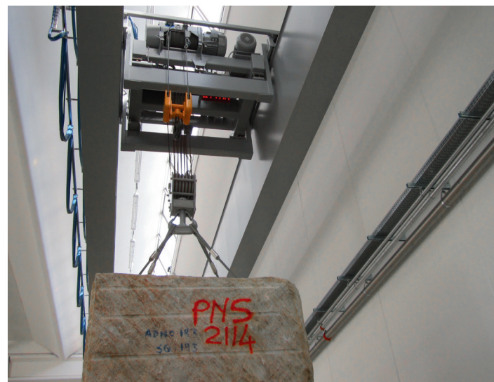
Detail of lifting trolley with weighing device
