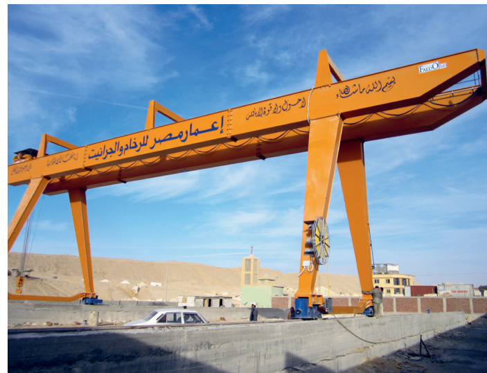
Gantry Crane, capacity 50 ton, span 20 m, lateral leaps 6 m
