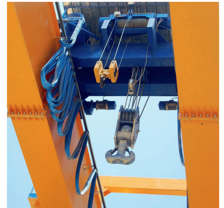
Detail of lifting trolley with auxiliary hoist
