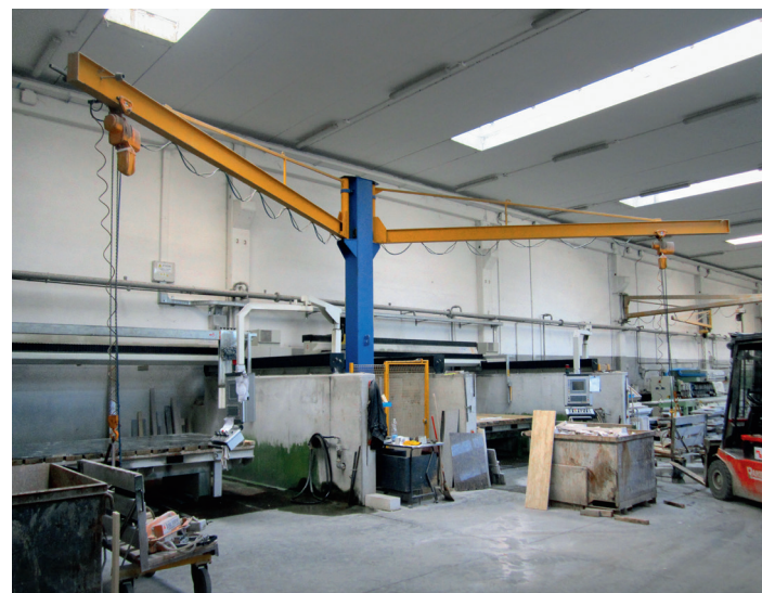
Jib Crane column mounted, capacity 1000 kg
