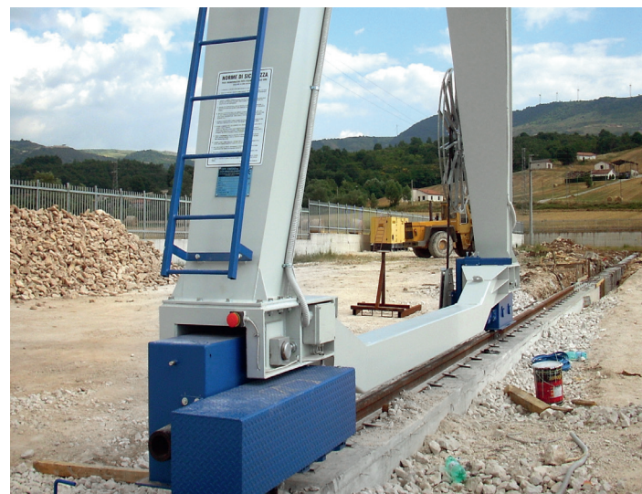
Detail of longheron and little trolleys
