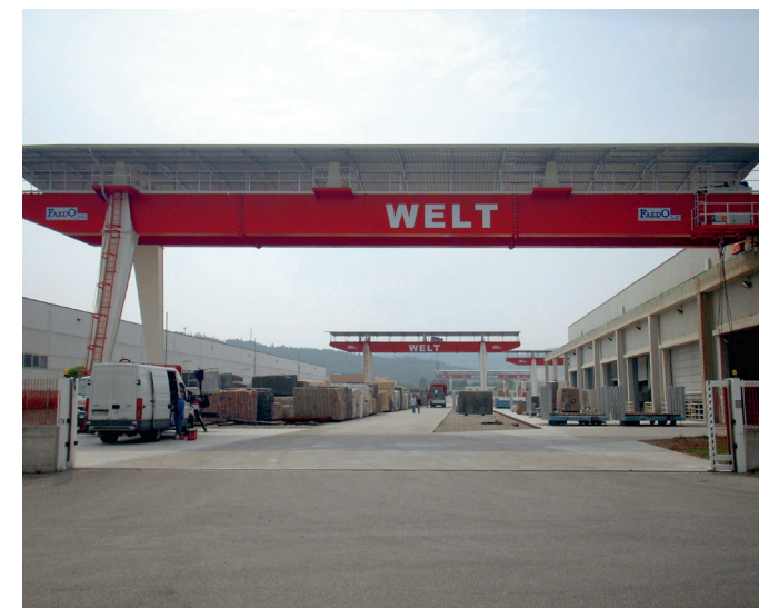
Hal Crane, capacity 40 ton, span 30 m, lateral leap 6 m
