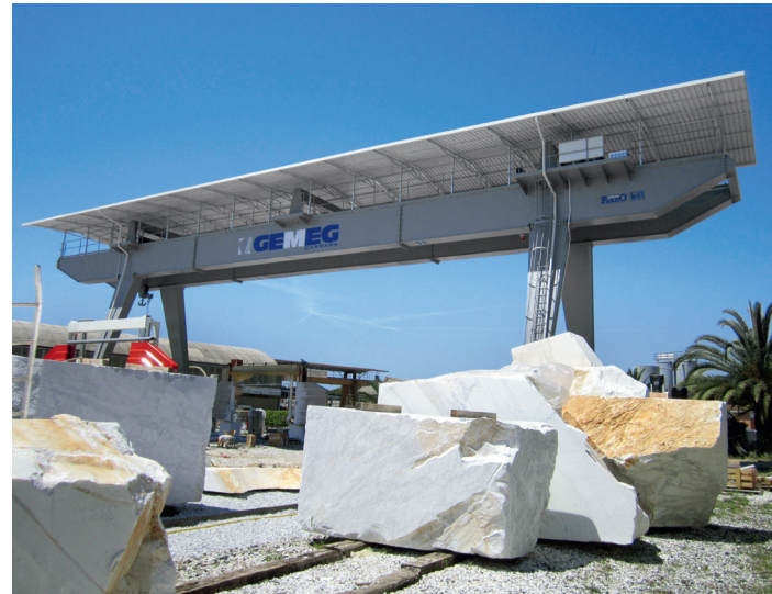
Gantry Crane, capacity 45 ton, span 25 m, lateral leaps 6,5/7,5 m
