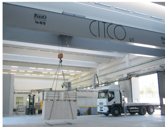
Overhead Crane, capacity 40 ton, span 20,9 m
