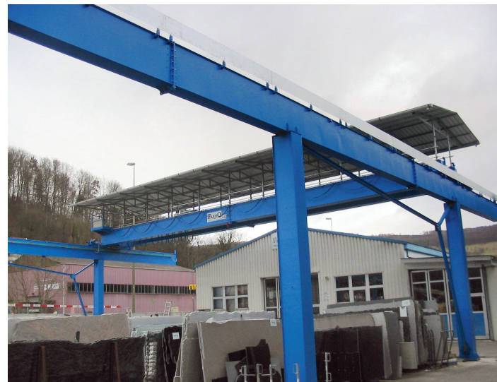
Overhead Crane, capacity 6,3 ton, span 23 m
