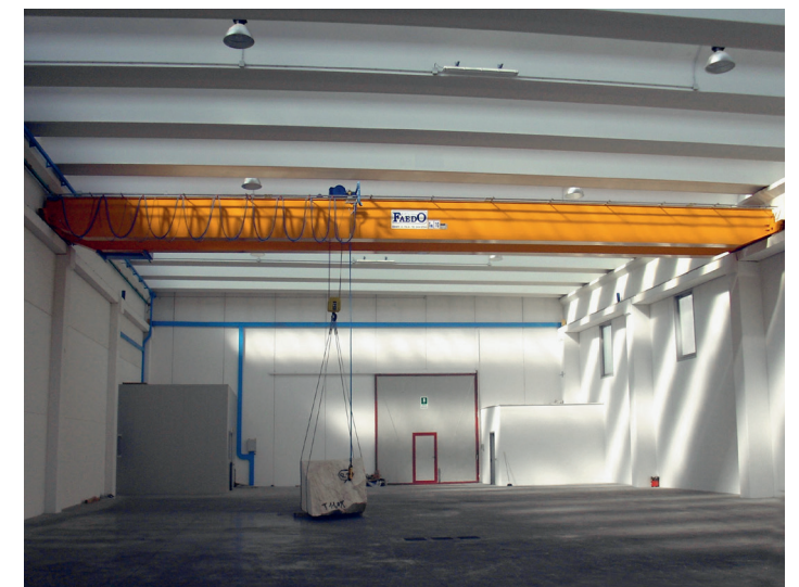
Overhead Crane, capacity 10 ton, span 20,7 m
