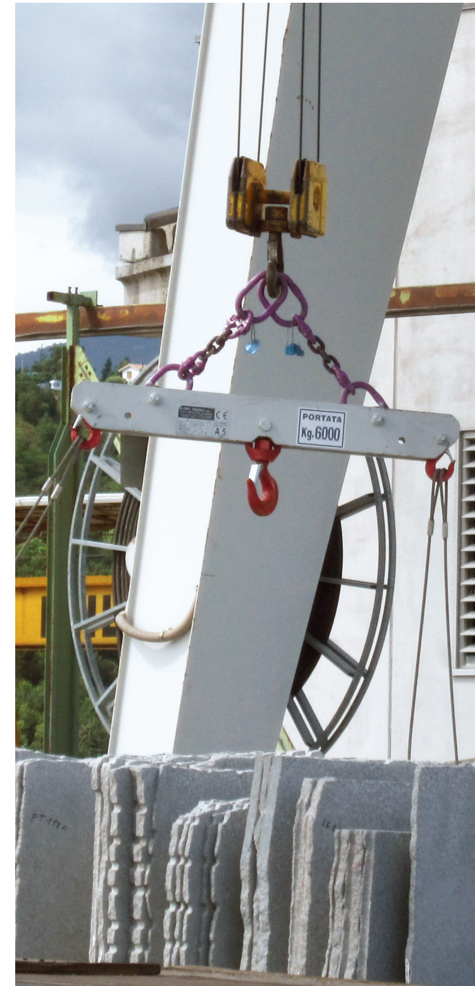
Sling beam capacity 6 ton
