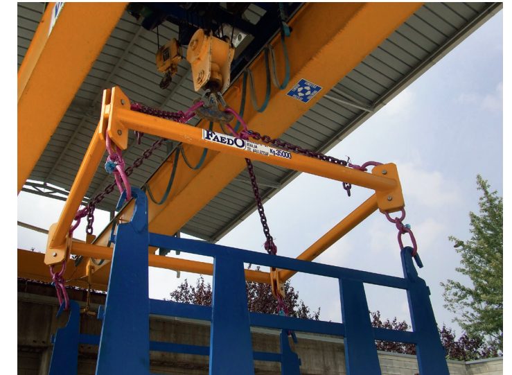
Sling beam for slabs and blocks, capacity 35 ton
