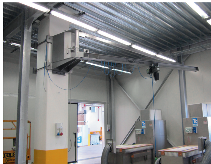
Jib Crane wall bracket mounted, capacity 1000 kg
