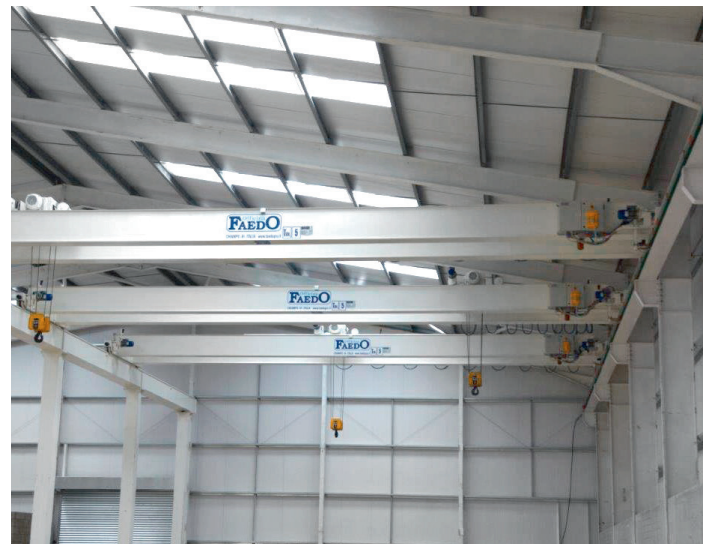
Overhead crane, capacity 5 ton, span 14 m
