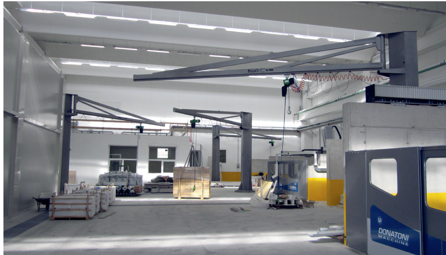
Jib Crane column mounted, capacity 1000 kg
