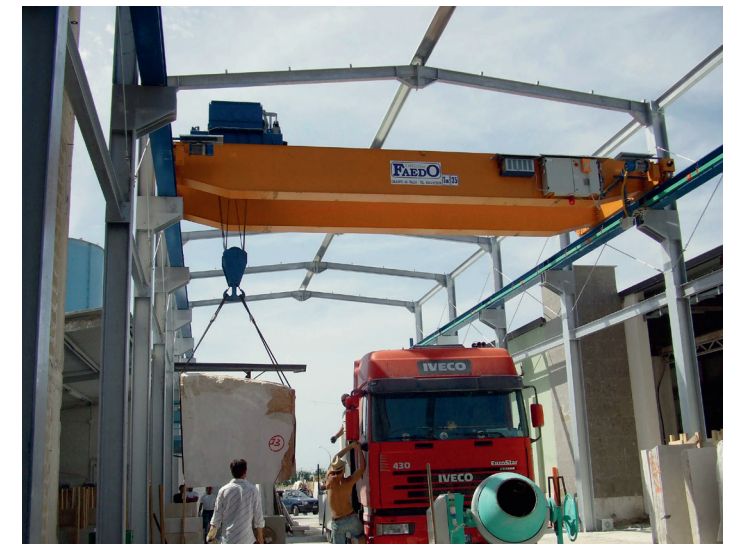
Overhead Crane, capacity 35 ton, span 10 m
