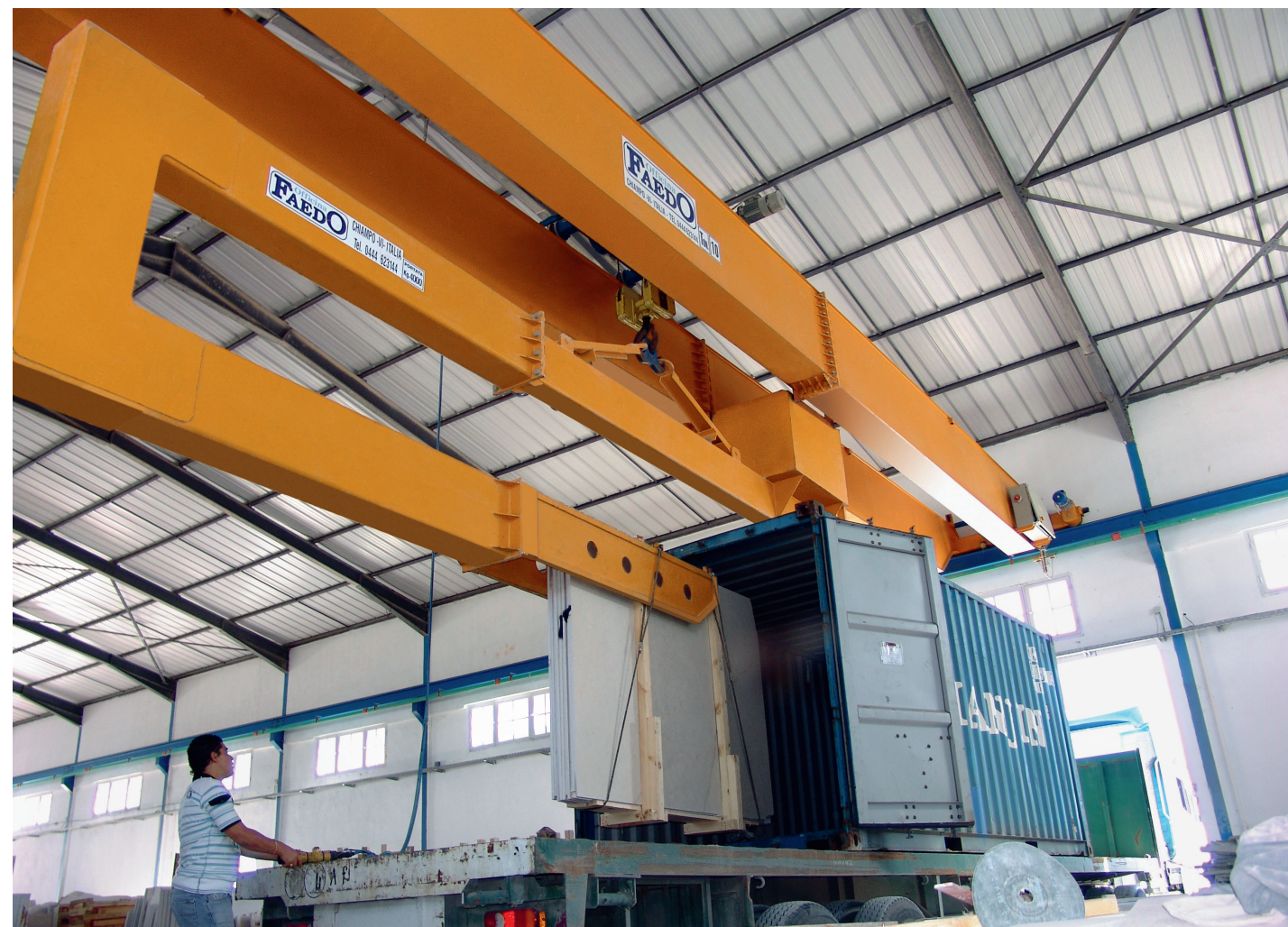
Loading Arm capacity 4000 kg
